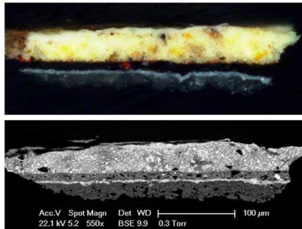
*Stratigraphic cross-section of a sample of the original yellow paint material (cross of Saint Nicolas) examined under an optical microscope (top) and under a scanning electron microscope (bottom). Visible between the deepest part of the ground and the paint layers is a fine layer of priming coat consisting of lead white.*
