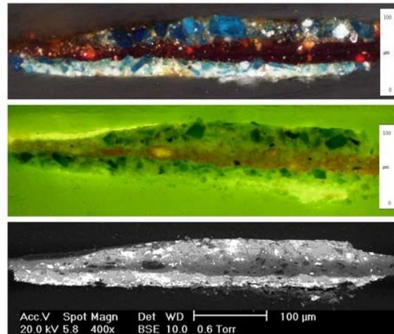
*Stratigraphic cross-section of a sample of the original blue paint material (mantle of the Virgin) examined under an optical microscope using direct light (top), using ultraviolet fluorescence (middle) and under a scanning electron microscope (bottom). Succession of glazing layers on the surface of the paint layer. From bottom to top: mainly azurite with lapis lazuli; red lacquer; mainly lapis lazuli with azurite.*
