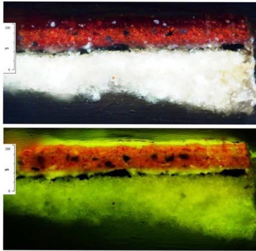
*Stratigraphic cross-section of a sample of the original red paint material (dark red of the cloak worn by Moses) examined under an optical microscope using direct light (top) and using ultraviolet fluorescence (bottom).*
