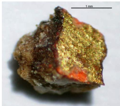
*Photograph through a stereoscopic microscope (30x) of a small sample of gilding on mordant taken from an angel. Left edge of the right compartment of the arched top.*
