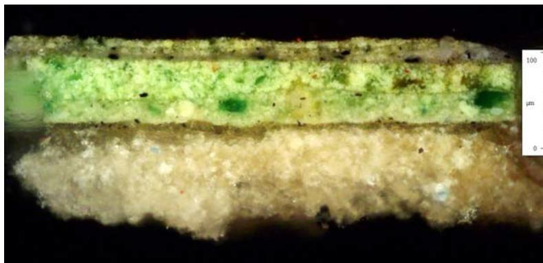
*Stratigraphic cross-section of a sample of the original pale-green paint matter examined by optical microscopy. White gypsum-based preparation (gesso), covered by several green-coloured layers applied using the glazing technique.*
